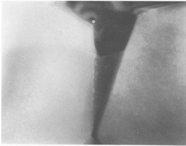
Figure 1 TEM micrograph of the as-received material showing the amorphous and crystalline intergranular phase surrounding the hexagonal silicon nitride grains ( \times 100\,000 ).
